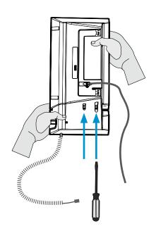
Connect the handset to the handset base, and connect the handset cable.
